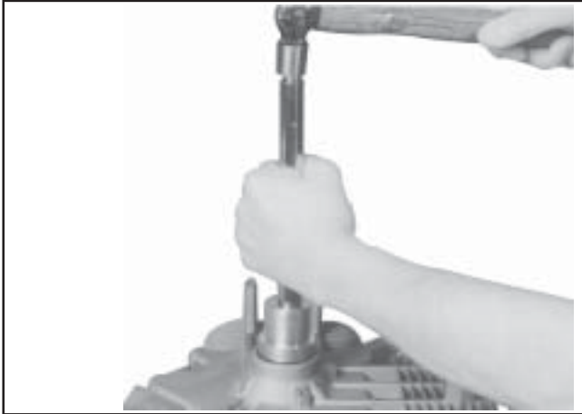
Figure 11-2. Installing Oil Seal in Crankcase.
